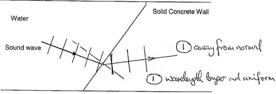
a) Draw a wave front diagram for a possible path of the sound wave as it refracts into the concrete.
