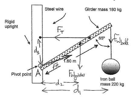
An iron ball of mass 220 kg is suspended from the end of a rigid steel girder.
