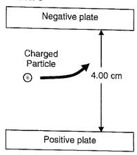
A charged particle enters a region between 2 parallel charged plates. The plates are separated by 4.00 cm. The electric field strength in the region between the charged plates is  $8.75 \times 10^4$  V m<sup>-1</sup>.
