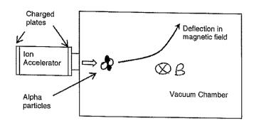
a. Calculate the potential difference between the charged plates in the Ion Accelerator that will give the alpha particles a maximum velocity of  $3.40 \times 10^5$  m s<sup>-1</sup>
